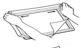
**Step 1** - Lay the frame onto a flat surface, tape side up, and remove the double sided tape from all 4 sides of the frame.
