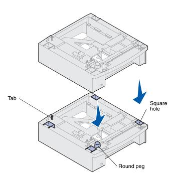
Place the support unit on top of any previously installed paper drawers, or the table or printer cabinet where you plan to use the printer.
