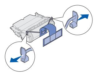
**c** Pull on each end of the plastic, V-shaped piece and then pull the packaging material straight out. Discard all packaging material.
