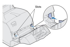
**3** Align the tabs on the envelope feeder with the slots on both sides of the printer, and then gently push the envelope feeder into the opening until it *snaps* into place.
