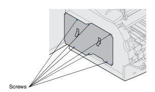
4 Loosen, but do not remove, the six screws on the shield.
