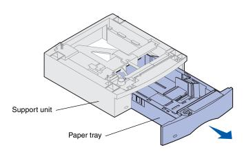
1 Remove the tray from the support unit. Remove all packing material and tape from both the support unit and the tray.
