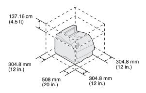
1 Select a well-ventilated place to set up your printer. Allow at least as much space as shown in the illustration. Make sure you have a sturdy, low table or the optional printer stand on which to set the printer.
