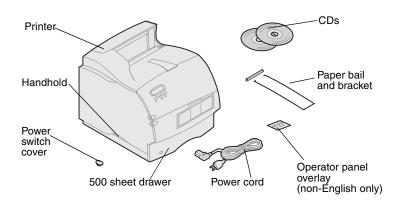
2 Remove all items from the box except the printer. If any items are missing, contact the place where you bought the printer.
