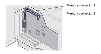
**Warning!** Electronic components can be damaged by static electricity. Touch something metal on the printer before you touch the memory option.
