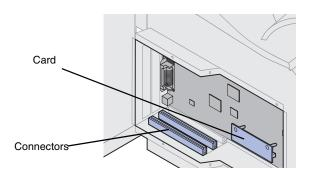
**3** Hold the firmware card by its edges, and align the two pins on the card with the holes on the system board.
