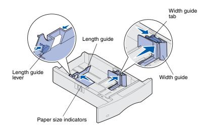
Complete these instructions to load print material into any of the standard or optional trays. All paper trays are loaded in the same way.
