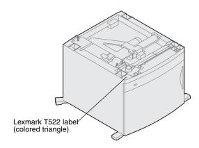
Your printer supports one 2000-sheet drawer. It gives your printer added capacity by letting you load up to four reams (approximately 2,000 sheets) of 20 lb. paper.
