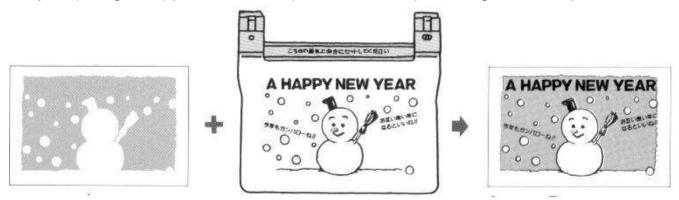
Using the printing example in Section 3-4, the second Print Master is inserted into the PG-11 and the artwork removed ready for printing. (*continued next page*)
