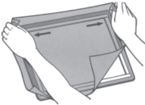
2. With the rough surface facing down, attach the screen to the frame. Start with one of the two longer sides.
