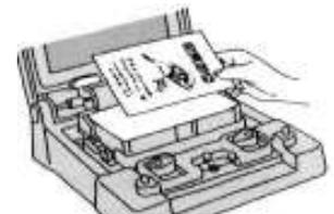
8. Close the lid and view the artwork through the stage glass – open and re-align if necessary.
