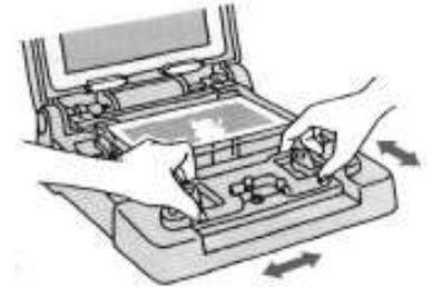
6. Adjust the Pad Table as necessary to align the print on the Registration Plate with the artwork underneath. Once you have aligned your design, tighten the Registration Pegs.
