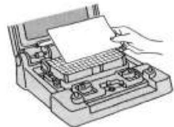
7. Lay you artwork on top of the card – ensure it is correctly aligned against the Paper Guide.
