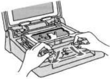
5. Lift the Lid of the PG-11 and gently peel off the Registration Plate from the back of the Print Master - it will stick because of the wet ink. Lower the Registration Plate over the Pad Table and loosen the Registration Guides.
