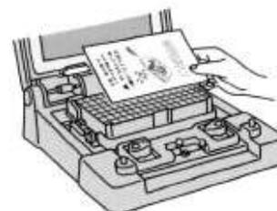
6. Insert card/ paper into the PG-11 using the Paper Guide to register for each print.
