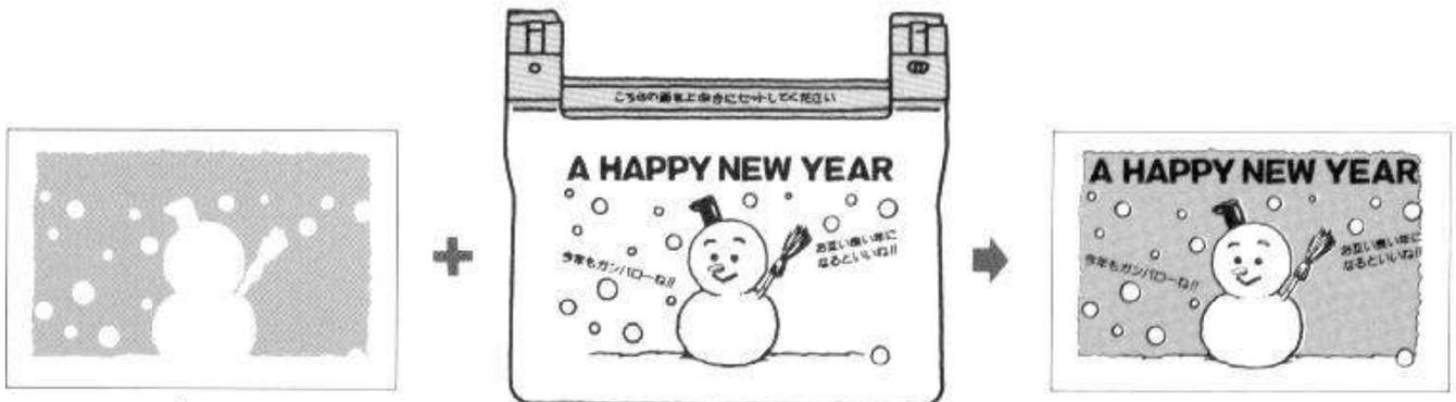
Using the printing example in Section 3-4, the second Print Master is inserted into the PG-11 and the artwork removed ready for printing. *(continued next page)*
