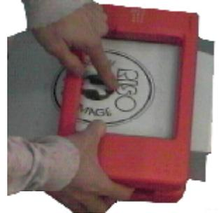
**4.** With your screen moved through the machine ready for the next section, insert new Print Lamps into the Lamp Housing and perform the imaging process again as details in **Section 3-1**
