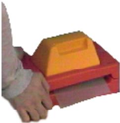
9. Lower the Lid of the machine and place the palms of your hand onto the front corners and press down to 'flash' the machine, imaging the design to the screen
