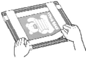
2. Leaving a 2 cm. wide border around the outside of the design, cover the outside area of the screen with Screen Masking Tape [T36]. Attach the tape to the back of the screen - film side of the ScreenMaster.
