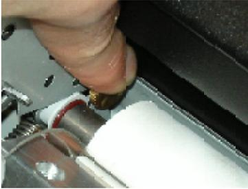
At the rear of the white rubber roller there are two clips which MUST be loosened before use. These clips are used in production and for transporting the machine.
