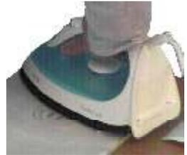
Note: Do not heat for longer than 2 seconds per pass as this will overheat the carbon
