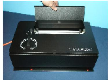
⇒ This will expose the glass roller, with the heat element inside, along with the white rubber roller at the back
